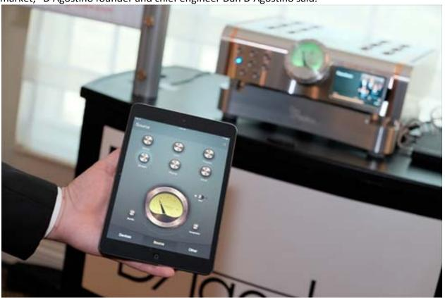
MLife uses the exact same amplifier and preamplifier circuits as the Momentum integrated amp, except that the integrated amp's tone controls have been replaced with a wired/wireless network interface. The network capability allows access to a practically unlimited amount of music and other audio content:
